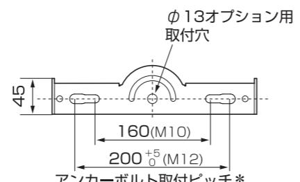
\* M12 anchor bolt case: mounting pitch 200mm
