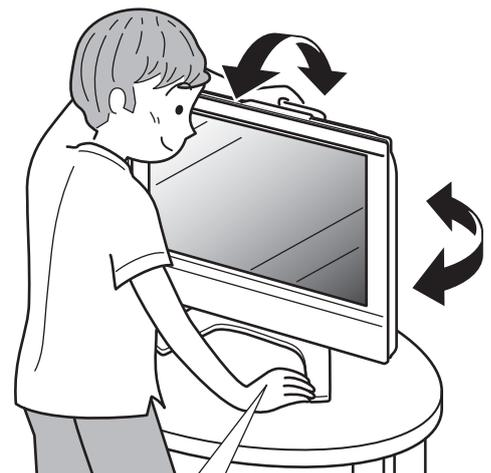
Hold the carrying handle and tilt the screen while steadying the stand with your other hand. The screen can be tilted up to 2.5° forward and 10° backward, and rotated horizontally up to 25° clockwise and counter-clockwise.
